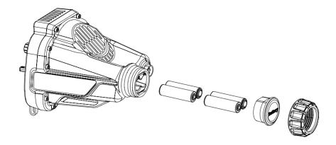
The Au GOLD FINDER is supplied with four AA Alkaline batteries.
