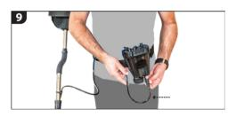
9. Pull approximately 14" of Au GOLD FINDER Coil Cable through the Flexible Belt Loop and attach Coil Cable Connector into System Box Cable Connector. Ensure Connectors are properly aligned and hand-tighten.
