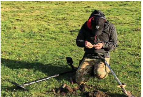
Having a higher Discrimination setting means you may not know what you have walked over. For example, you're on a new field and you set Discrimination to 09. You only hear the good solid targets (non-ferrous), because you can't hear the iron you could be walking over and iron could potentially mean a site with nails which is an indication of habitation.
