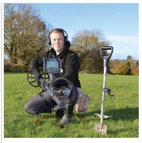
omits as it has very fast reactivity. This will help to distinguish any tiny targets close to iron. If you get a mixed signal, they're always worth investigating as the Anfibio is a VERY FAST machine and it's telling you that two targets are present. If you hear a grunt, but also a beep mixed into the signal, it could be an indication that there are two targets next to each other. I always say - IF IN DOUBT DIG IT OUT!
