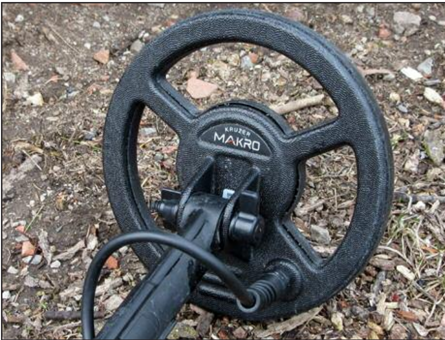
The 7" KR18C has surprising depth for a small coil. In particular, it makes an excellent gold jewelry coil for the water's edge or busy sunbathing ground. The Anfibio's 20 kHz option gives it even more gold sensitivity.
