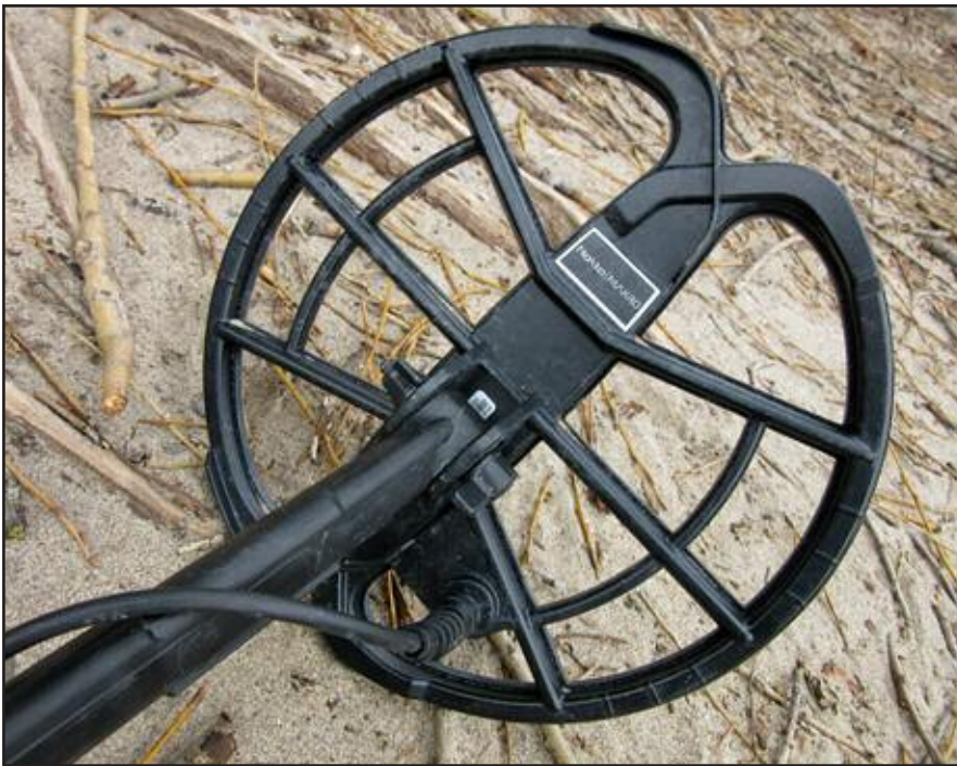
The Anfibio's new 11" Double D searchcoil had both great depth and razor-sharp separation in dense iron.
